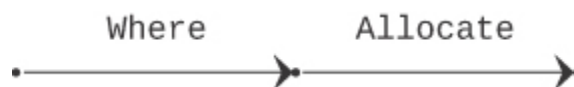
Figure 13.3 Sequential composition of two functions. The output from Where becomes the input to Allocate .
