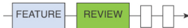
Figure 9.7 Reduce the wait time between feature completion and code review. A review will typically spark some improvements, and a smaller review of those improvements. These activities are indicated by the smaller boxes to the right of the review.
